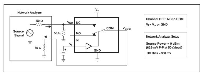
Figure 17. OFF Isolation (O<sub>ISO</sub>)
