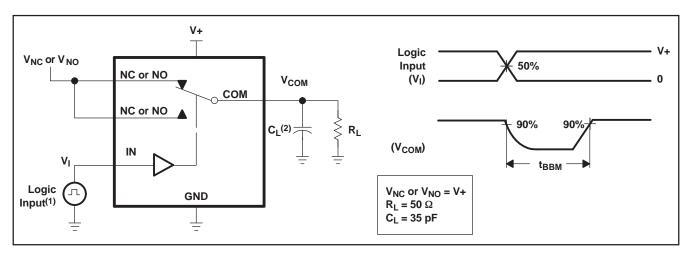
(1) All input pulses are supplied by generators having the following characteristics: PRR  $\leq$  10 MHz, Z<sub>O</sub> = 50  $\Omega$ , t<sub>r</sub> < 5 ns, t<sub>f</sub> < 5 ns.
