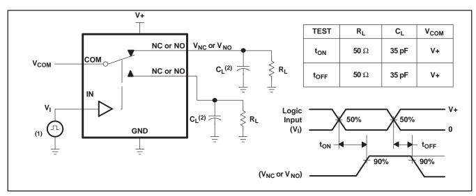
(1) All input pulses are supplied by generators having the following characteristics: PRR  $\leq$  10 MHz, Z<sub>0</sub> = 50  $\Omega$ , t<sub>r</sub> < 5 ns, t<sub>f</sub> < 5 ns.
