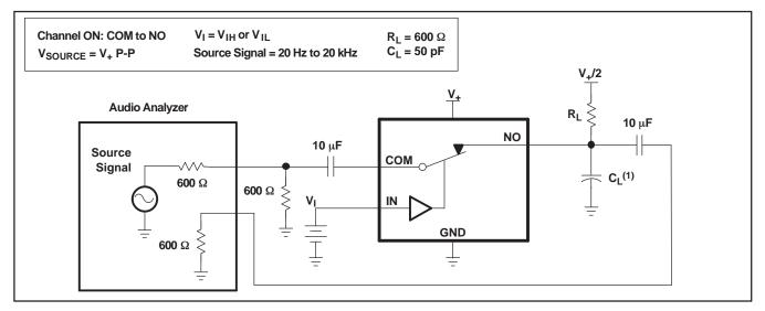
A.  $C_L$  includes probe and jig capacitance.
